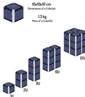
Figure 1. CubeSat Sizes and Configuration
