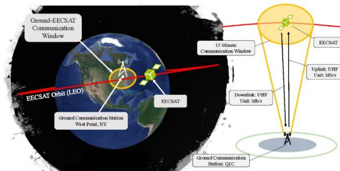
Figure 3. EECSat OV-1 Diagram
