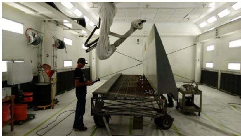
Figure 1. Robotic Painting Arm at WR-ALC
